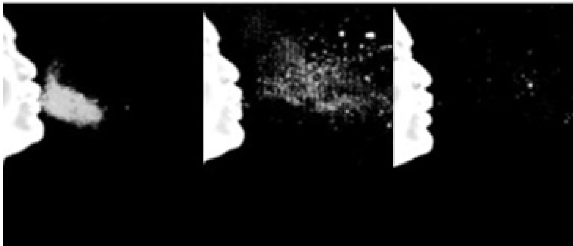
Image of droplets movement during cough period taken by PIV
